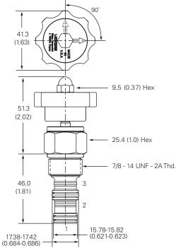
Torque cartridge in housing A - 47-54 Nm (35-40 ft. lbs) S - 68-75 Nm (50-55 ft. lbs)
