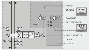
Selecting the CW-option allows user specific applications to be developed in Eaton's Pro-FX Control software tool, which is based on the popular CODESYS development environment.
