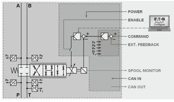
Level 3 valve integrated pressure sensors can be used for machine health monitoring with data broadcast over the CANopen bus or employed for pressure control in addition to the external motion control illustrated for the level 2 valve.
