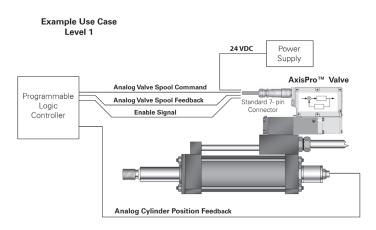
AxisPro level 1 valves, such as KBS1-03 (ISO size 3), can be used to control machine motions in open loop or closed loop control applications. The valve receives its analog command input on the 7-pin, main, connector from an external axis control device.
