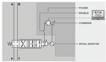
Centralized motion control, relying on external motion controller, not shown in the diagram
