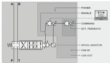
Distributed motion control, taking advantage of the available axis-control function embedded in the valve controller for AxisPro level 2 and 3.Command can be analog via the 7-pin connector or via CANopen using the M12 connections illustrated on page 12.
