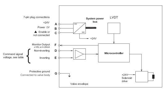
▲ Pin C is used for a valve enable signal with electrical connections Field 8 = H or R.
