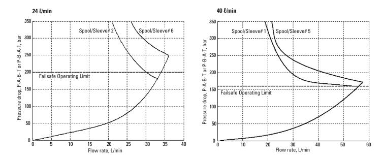
**Operating Limit:** When operating the valve beyond the operating pressure limit, spool may not return to failsafe when power is removed
