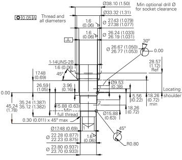
Note: Tightening torque of "F" adjuster locknut - 20 to 25 Nm.
