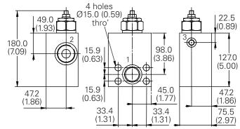
Note: For applications above 210 bar - please consult our technical department or use the steel body option. Note: Tightening torque of "F" adjuster locknut -20 to 25 Nm.
