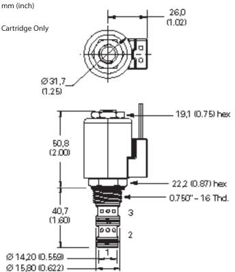
Torque cartridge in steel or (25-30 ft lbs)
